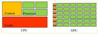
The GPU's hardware configuration makes it perfect for graphics processing, where the same compute-intensive calculations are performed on very little data. Another aspect of the GPU's graphics origins is that it does not support highly accurate calculations because it uses single-precision. The low-memory requirements of graphics also make the amount of cache limited. Below is a more detailed image of the types of memory on a GPU.
