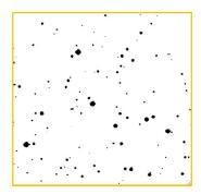
To further clean the image, a blurring reduction technique is used in which a 9 by 9 window is created around each pixel in the binary image. Then, the median value of these 9 pixels is taken. If the median is 0, then the center pixel is set to black. If the median is 1, the center pixel is set to white (remember the image is inverted, so stars are black). The resulting stars are much more defined and clearly separated.
